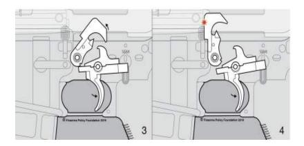
In a semiautomatic firearm, the bolt re-cocks the hammer. By the time the bolt reciprocates, the operator may still have the trigger depressed. This is where the "disconnector" comes into play. When the trigger is depressed, the disconnector moves into its active state. Image 5. When the weapon fires, the bolt travels rearward, pushing the hammer to the rear. The disconnector captures the hammer near its rearmost position. Image 6.
