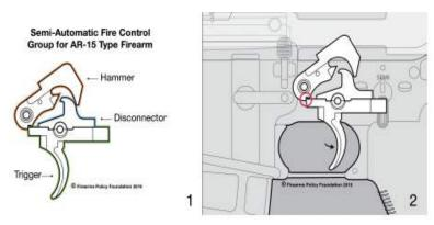
The hammer is spring-loaded, storing energy as it is moved rearward into the "cocked" position. The trigger keeps the hammer in the "cocked" position by way of its "sear," a geometric plane that locks the trigger and hammer together. Image 2. When the trigger is depressed, the trigger sear slides out of the way of the hammer, allowing the hammer to swing and strike the firing pin. Image 3.
