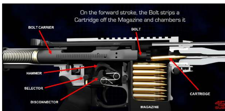
Figure 2: Post-Fire Forward Motion of Bolt Carrier 9
