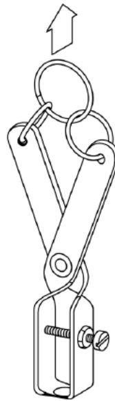
Figure 11 to paragraph (k)(3) - Tension Test Adapter Clamp
