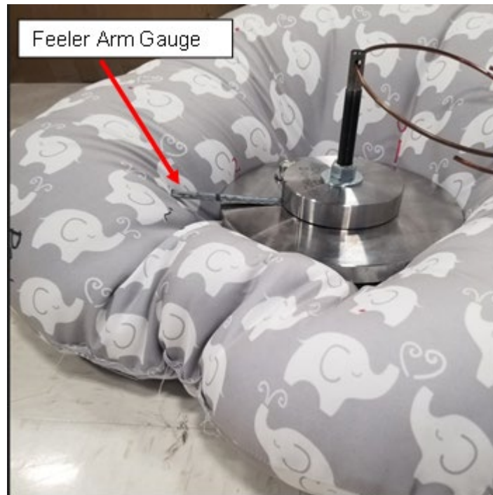
Figure 5. ASTM OSS Test with 8-in Diameter Probe, Sample 240
